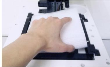
⑤ When the platform is moved to the top, remove the protecting foam.
