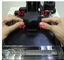
Tighten the screws with fingers. First tighten the front screws. Fasten screw F1 then F2. And tighten the screws at the back. Fasten screw B1 then B2.
