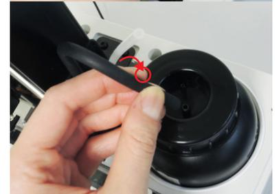
⑪ Push the tubes all the way down. First attach the black tube to thick nozzle, and then connect the transparent tube to thin nozzle.
