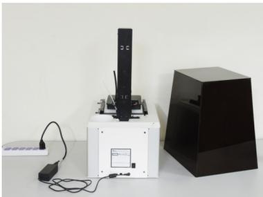
② Connect power adapter, power cord to the printer.
