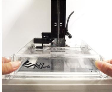
⑥ Unpack the resin tank and insert it into the tank slot. Push all the way until reaching the end.
