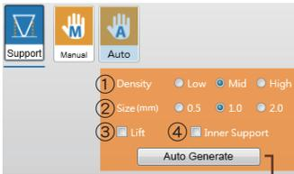
**Support auto generation:** XYZware\_Nobel is able to analyze the features of the model and add support structure to where necessary. Simply select a desired density <sup>①</sup> and size <sup>②</sup>, choose to "Lift" <sup>③</sup> the print and/or print without internal support <sup>④</sup>, and press "Generate" to preview the support structure.
