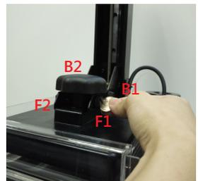
Finally tighten the screws with a coin or other tools (sequence from F1, B1, F2 to B2) and press [OK] to complete calibration.
