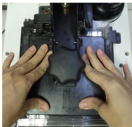
When you see the message above, press the platform with both hands 3 times. Make sure you see the right side of the tank sinks into the tank slot slightly.
