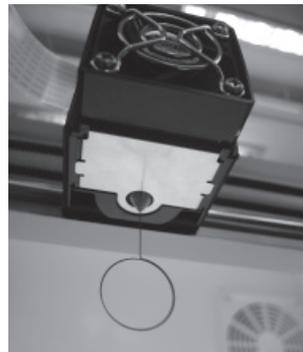
3. Hold the cleaning wire with the pliers, and carefully pass the wire through the nozzle opening.
