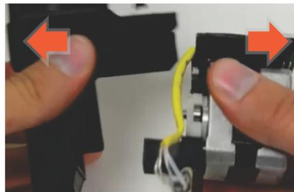
Using the Alan key tool, unscrew the white gear cover (2 screws). Then pull the gear cover off the motor (snap lock). Remove the plastic dust residue from the gear and clean the surrounding area.
