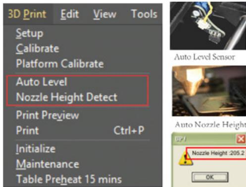
The most important part of 3D printing is having a level platform and the correct distance between the nozzle and the platform. Click "**Auto Level**", the head will check 9 points around the platform are level, then it will set the platform/nozzle height.
