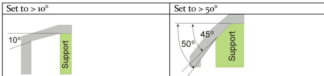
There is always a delicate balance between minimizing the amount of support material, versus the quality of the part, versus the difficulty of removing support material.
