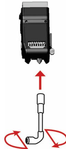
**TIP:** To keep your prints looking great it is important to keep the outside of your nozzle clean and free from leaving dark blotches in your prints. Always keep your nozzle clean. Do a withdraw and once at temperature (*beep*) give the nozzle a wipe with a piece of old denim jeans (non synthetic).
