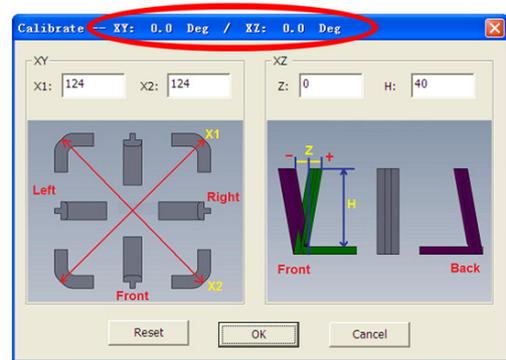
The Vertical calibration procedure allows you to ensure that the printer platform is perfectly horizontal and that the printer prints consistently in the X, Y and Z direction.
