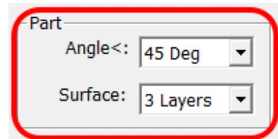
**Stable Support:** Stable support creates support that is rigid and the model is less likely to distort, but the support material is more difficult to remove.
