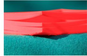
You absolutely must not open the UP BOX doors during printing, as it is as bad for the ABS as it would be for opening the oven when making Soufflé. A sudden rush of cold air can warp or split your model.
