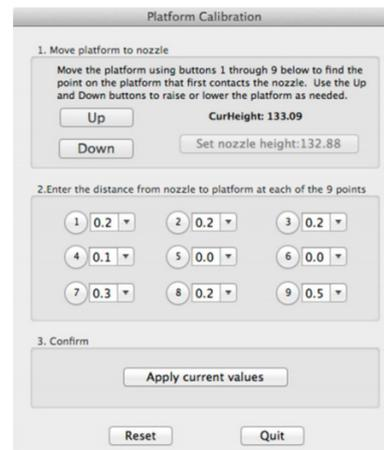
The values in the image above indicate that the print surface is warped, with the center higher than both the front and back edges.
