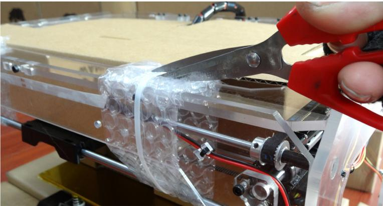
A. Use strong scissors or a wire cutter to cut the zip ties holding the gantry system in place. Discard the zip ties and the plastic pieces holding them in place.
